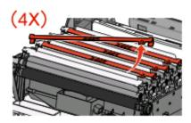
Remove the red packing strip from the top of each photoconductor.
