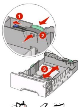
Squeeze the length guide tabs together, and then slide the guide to the correct position for the size of paper being loaded.
