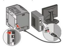
**7** Connect the power cable to the printer and then to a properly grounded electrical outlet, and then turn the printer on.
