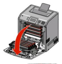
Allow the front door to open completely.
