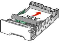
Load the paper stack with the recommended print side faceup. Load the stack toward the back of the tray as shown.
