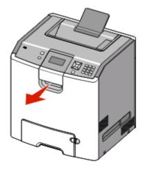
Grasp the handle, and pull forward to open the front door
