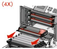
Pull each toner cartridge straight out of the printer, one at a time.
