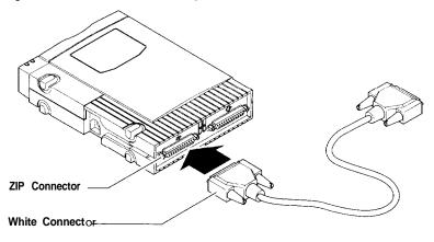
Connect the other end of the cable to your computer s parallel port (printer port). (If a printer is connected to the only parallel port, disconnect it and use pass-through feature described in Step 5.)
