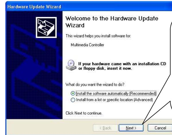
Turn on the computer, Windows will auto detect new hardware. Insert the CD and press “Next”. The installation will auto find the driver in the CD
